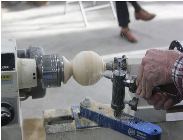
Tom Hurst's Sphere Construction
