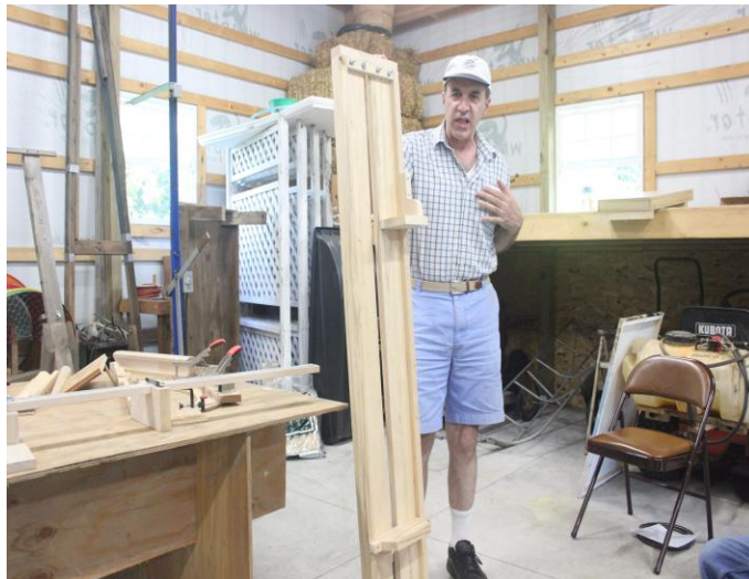
John DeLapa's Sawmill Jig for Bandsaws
