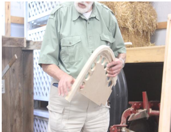
John Harsh's Jig for Making a Canoe Stern Stem
