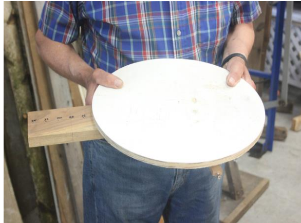
Roger Bredeveg's Jig for Cutting Circles With a Bandsaw
