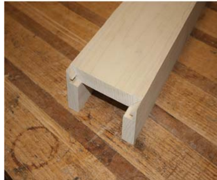
Jim Woodfin's Lock Miter Bit and Joint Example
